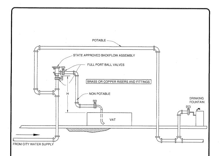
"H" MINIMUM HEIGHT OF UNIT SHALL BE 12" ABOVE HIGHEST FLOW LEVEL, RIM OF TANKS, VATS, OR BASINS. (SPECIAL CONDITIONS MAY REQUIRE MORE HEIGHT)
