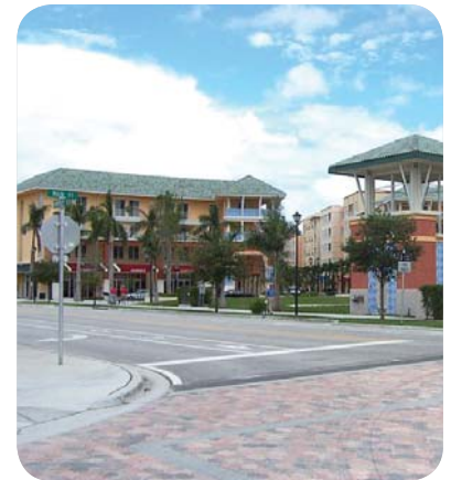
The vehicular zone can be enhanced through design techniques such as special paving.
