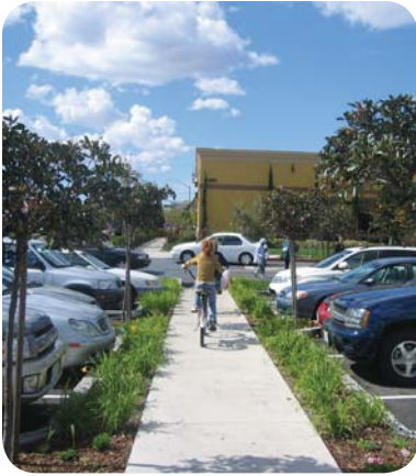
Parking lot landscape islands should have be a minimum curb to curb width of five feet wide to accommodate landscaping and sidewalks.
