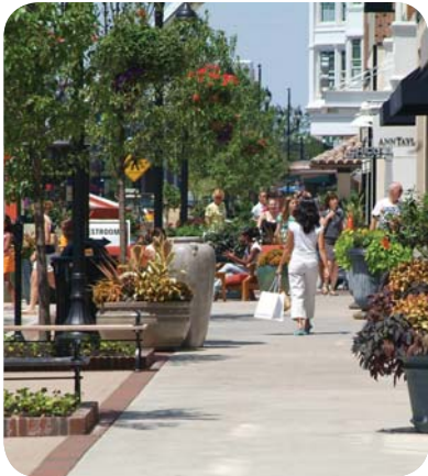
A minimum 8-foot-wide unobstructed pedestrian walkway shall be provided on Bolsa Avenue.
