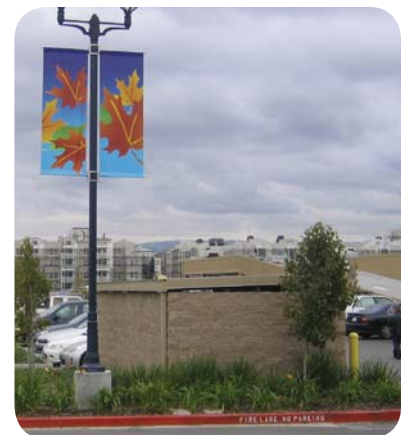
Trash enclosures located in parking lots should be separated from adjacent stalls by planters.
