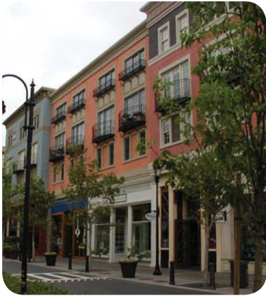
The use of horizontal bands and ornamentation on the building facade can help reduce its bulk.
