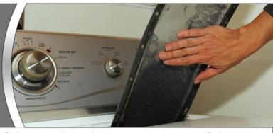
The leading cause of home dryer fires is failure to clean them. Fires can occur if there is a build-up of lint in the dryer or the exhaust duct. Lint can block the flow of air which can cause excessive heat build-up, resulting in fire.
