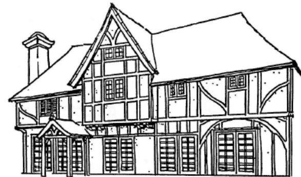
Typical example of half-timber cross bracing
