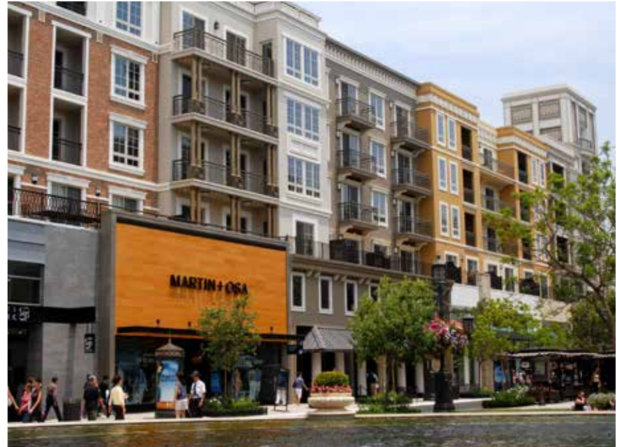
Façade articulation including notched setbacks, projecting bays, and balconies helps to break up building mass and add visual interest.
