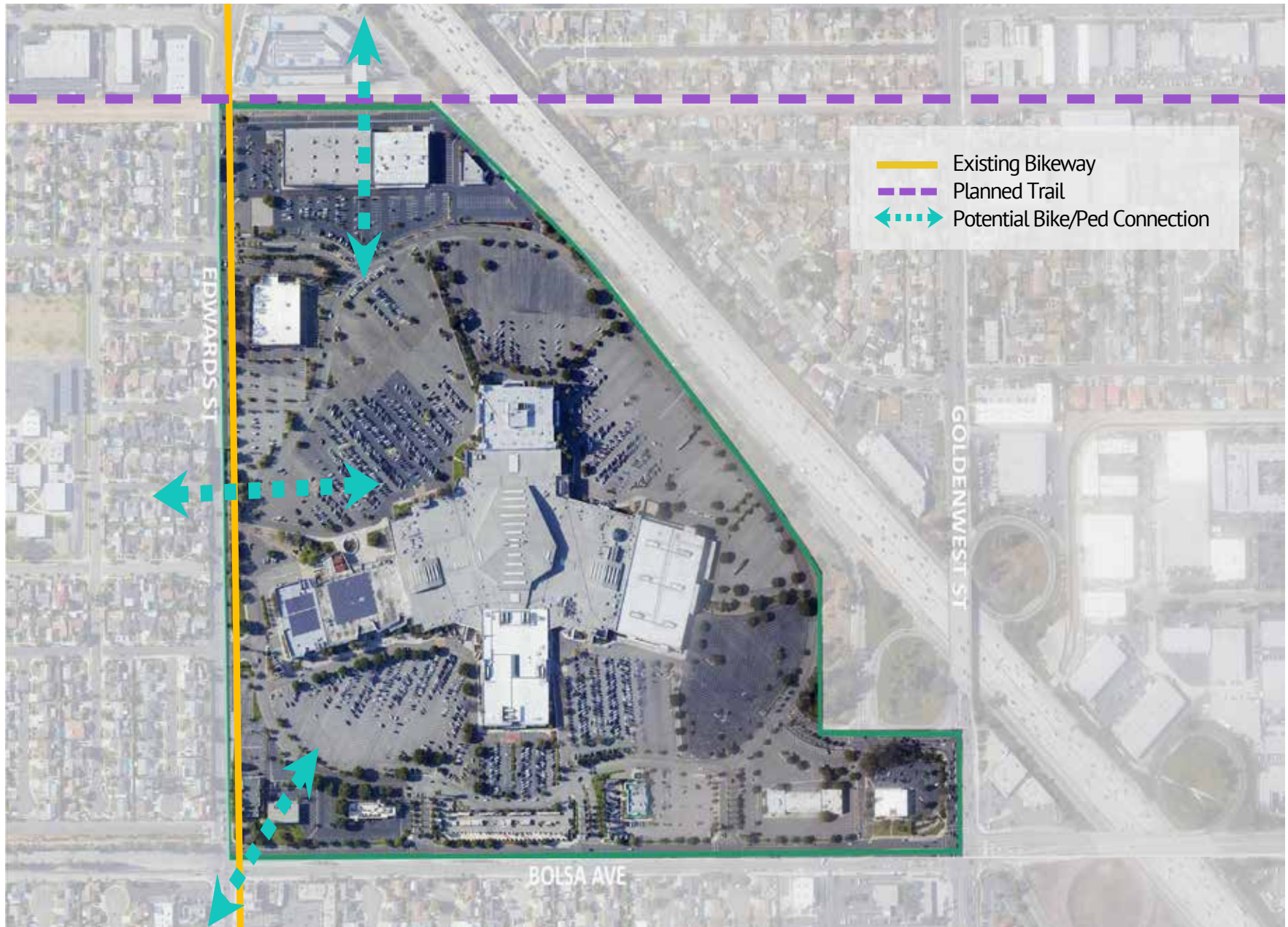
Figure 6.18: Bikeway and Pedestrian Improvements
