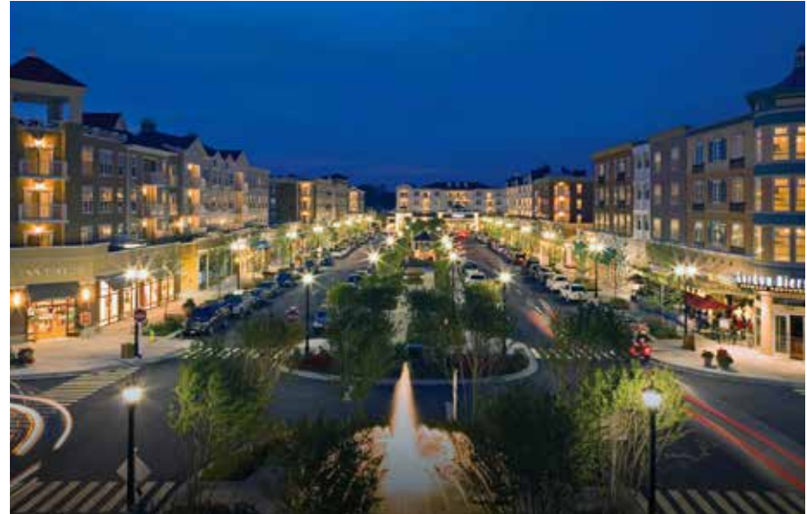
The photo above represents the implementation of Figure 6.8, Internal Main Street Section (Option 2). Parking going both directions is provided in a center median, which can also serve as a gathering space for Farmers Markets or other temporary outdoor events to help create activity in the project area.
